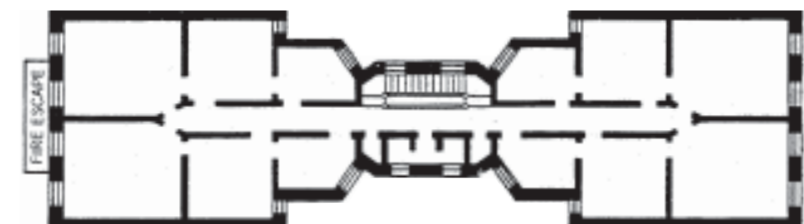
The dumbbell apartment layout was so named for the shape of its floor plan.
