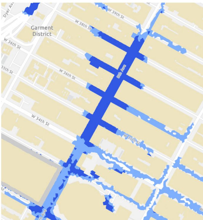
Map from NYC Stormwater Maps showing extreme flood conditions (3.66 inches/hour). Dark blue areas are deep and contiguous flooding greater than 1 foot deep.
